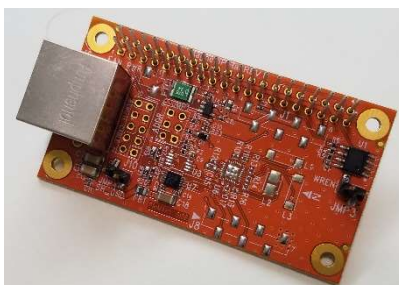
Local MagPi, header in place
