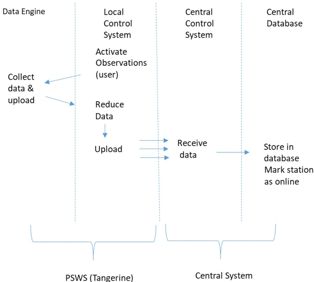
**Figure 4. Use Case 3, Local data reduction + continuous upload.**
