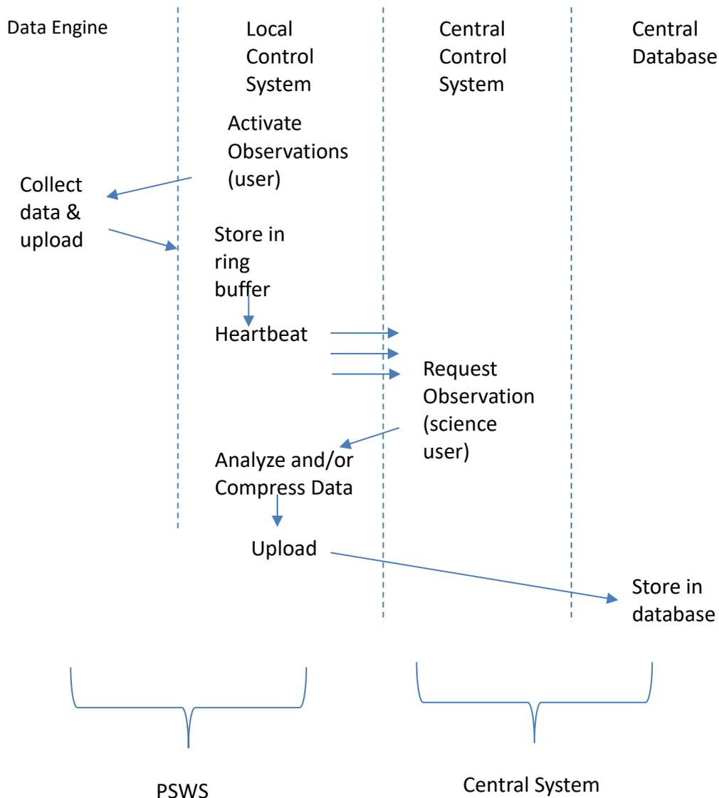
Figure 13. Use Case 1. Request/Response process model.
