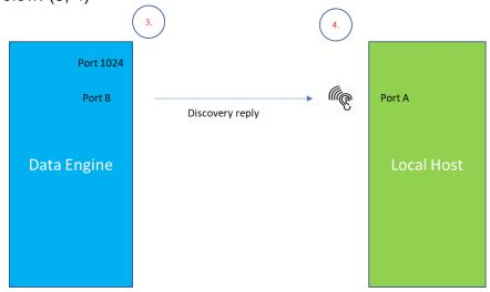
The DE responds; from this response, the LH learns the DE's IP address and provisioning port ("Port B"). • The DE now starts listening on its Port B. Port A – Port B form the **Provisioning Pair.** See Figure 3, below.
