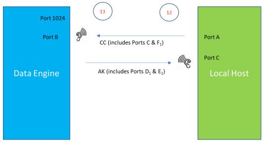
Assuming the DE is able to fulfil the request, it adds a second channel pair with AK, as shown above. (12, 13) Now, we have two channels that are independently controllable; Figure 7, below.
