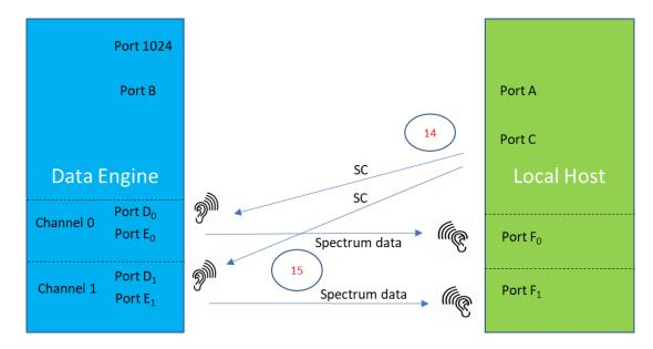
Each channel is numbered and can be started and stopped; when the LH wishes to delete a channel, it can issue the UC (Undefine Channel) command.
