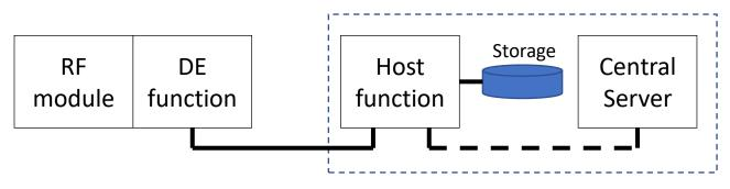
Implementation B: Host Integrated with Central Server. High bandwidth LAN from Data Engine to Processing.
