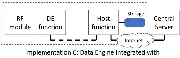
Host (e.g. FPGA with embedded CPU).
