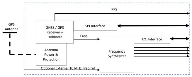
Figure 1. Block Diagram of Clock Module
